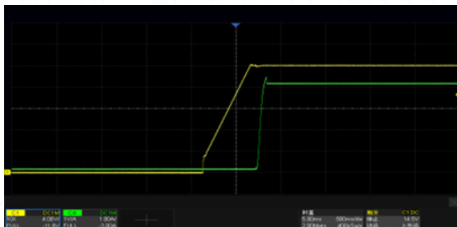
Figure 4-2(a). CC/CV Priority Mode Waveforms
